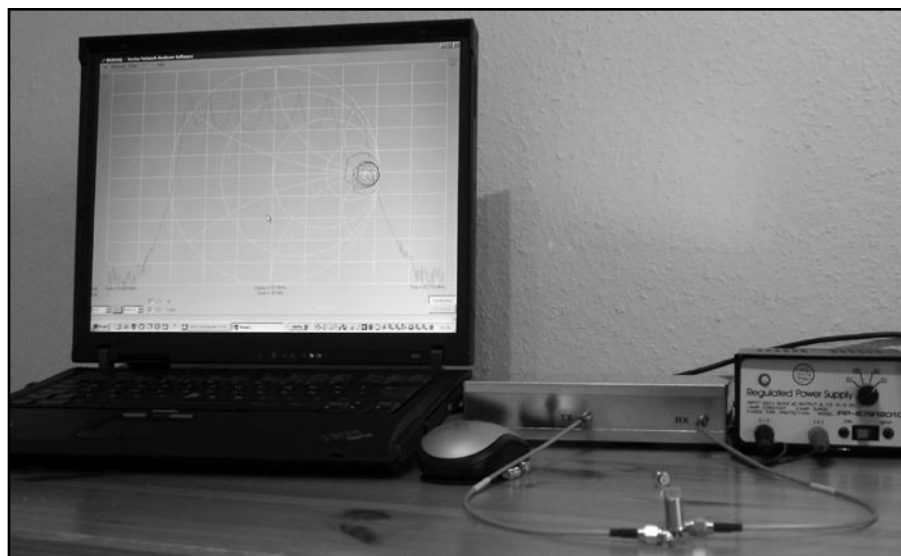
Figure 11 — Complete measurement setup with a monolithic crystal filter connected.
