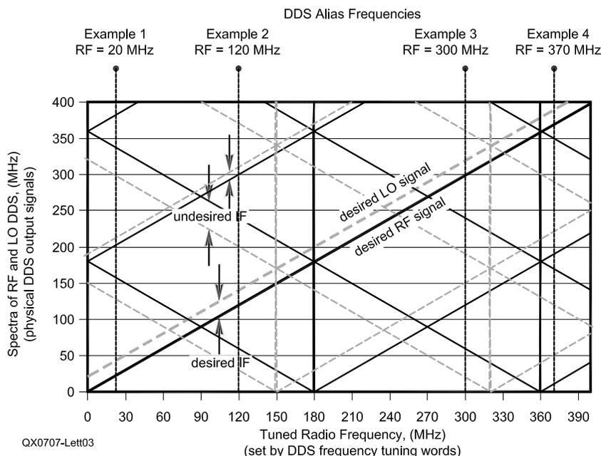
**Figure 3** — LO and RF DDS output spectra versus tuned RF. The solid traces are RF signals and the dashed traces are LO signals. The arrows indicate some possible RF-LO-mixing products. The examples are described in more detail in Tables 1-3. For better visibility, the RF clock frequency is 180 MHz, the LO clock frequency is 170 MHz and the desired IF is 20 MHz.
