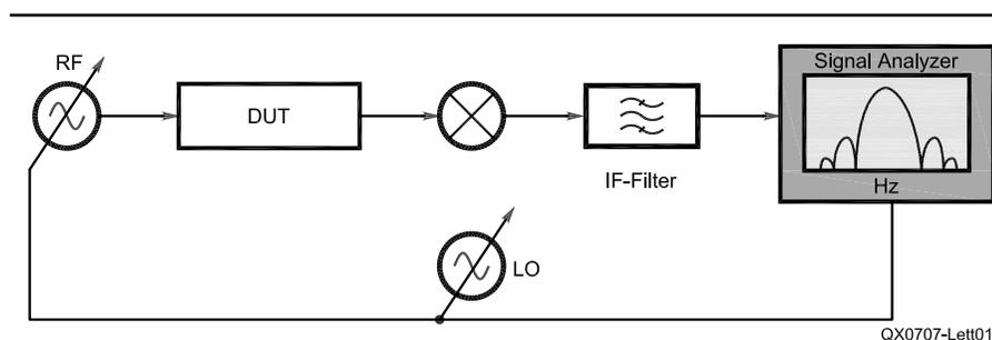
Figure 1 — Basic setup of a network analyzer.
