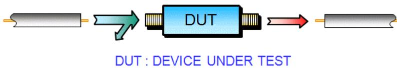
An electrical two port device behaves quite similarly, when inserted between two transmission lines, where the left one is guiding an electrical wave into the device. Some of the electrical power might get reflected at the device input (reflection loss), some will be converted into heat inside the device (dissipation) and the rest will come out of the device at the right hand side.
