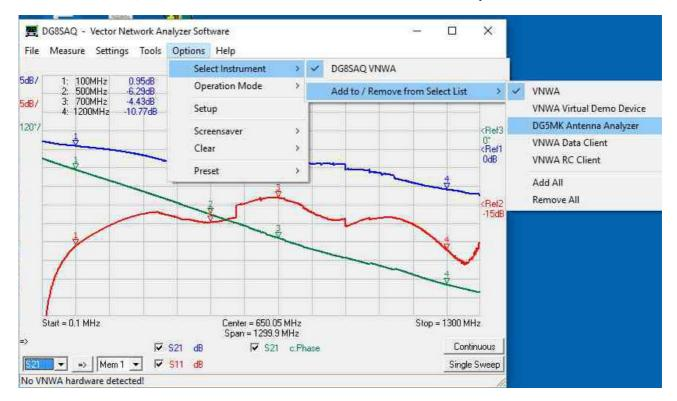
• Click on **Options** and **Select Instrument** once more and tick the box to select **the DG5MK Antenna Analyzer.**
