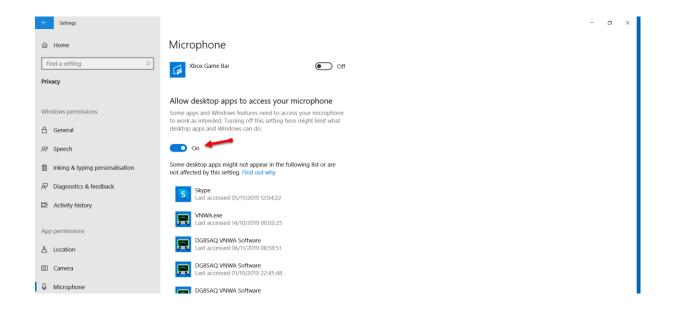
Close the window and restart the VNWA software. Now, VNWA should be able to access the VNWA USB sound chips.
