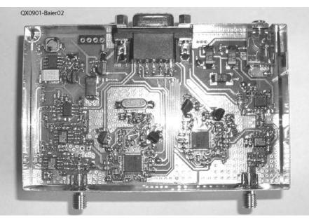
Figure 2 — Top view of the VNWA2.1 board. Board size is 100 × 60 mm<sup>2</sup>.
