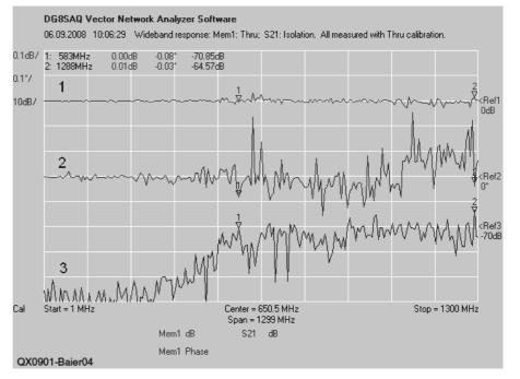
Figure 4 — Wideband transmission response of a through calibration standard from 1 MHz to 1.3 GHz obtained with dynamic clock multiplier adaptation during the sweep (trace 1 / Mem1-dB: amplitude response; trace 2 / Mem1-Phase: phase response) and wideband isolation (trace 3 / S21-dB). A through calibration has been performed prior to measurement.
