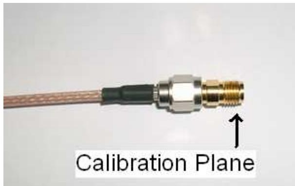
We select "Measure-Calibrate" or simply press the c-key on the keyboard, press the "Open" button, confirm that the open standard is connected and observe the instrument measuring the standard. When the measurement is completed, the red Open light turns green:
